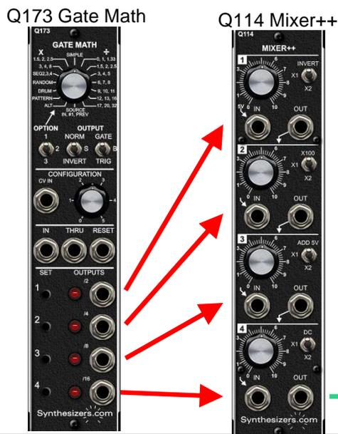
You don't have to use all 4 channels for sequencing. Use 2 for sequencing and 2 for mixing, or 3 for sequencing and 1 for amplification or inverting. Or 2 different sequences of 2 stages each.
