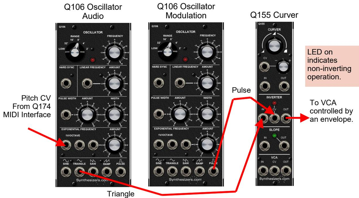
Use the inverter section to invert gate signals or envelopes. In this example, gate from a sequencer is patched through the Q155 and the gates polarity is controlled by a row of sequencer knobs.
