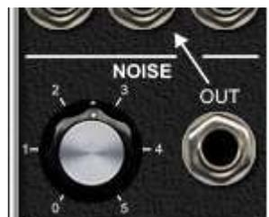
The knob controls a low-pass filter by default but can be changed to control noise level if desired.
