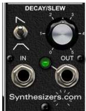
In the slew mode, without a plug inserted, the circuit loops automatically like an LFO to provide gates or modulation signals.
