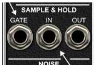
The Sample & Hold section gets its signal input from the Noise section. This creates a typical random stair-stepped signal source used for filter and oscillator modulation. To use a different signal, simply insert a plug to break the default connection.
